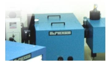
The Model 205f uses large 120 x 150-mm gratings to achieve phenomenal light gathering and throughput. The fast aperture ratio is excellent for low light applications, like Raman and photoluminescence. Any time photons are at a premium the Model 205f can help. It can be equipped with the 789A-3 digital scan control for scanning or with corrected optics for imaging applications.
